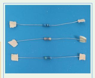
If your resistors do not have labels, work out which is which from the colours.
