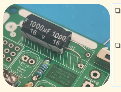
Bend the legs, as in the picture on the left. Attach to the board with the stripes lined up.
