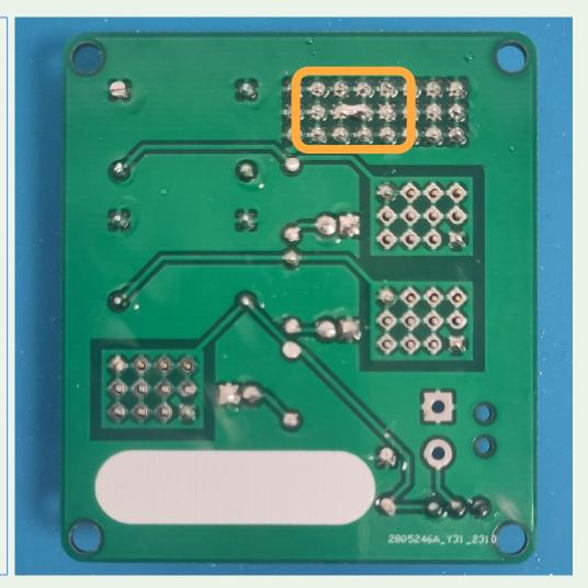
Solder your battery connector, with the metal parts facing outwards.
